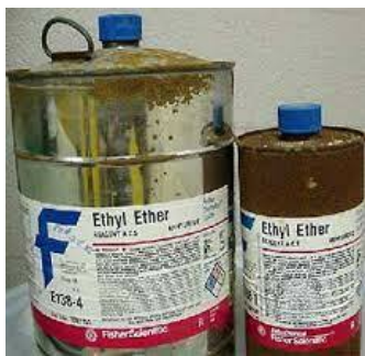
Ethyl ether is a Class B peroxide former that is common in laboratories
