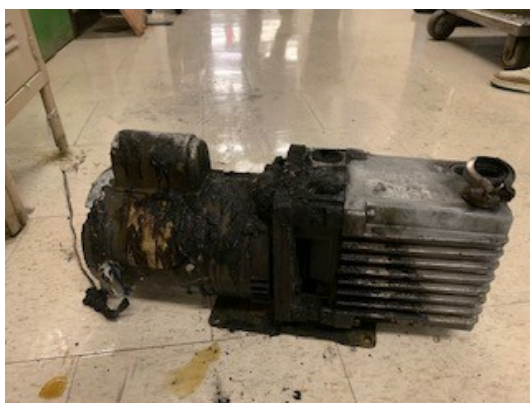
Penn vacuum pump after explosion
