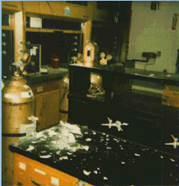
Figure 2. A second view of the fume hood involved in the fire. Notice the severe charring of the cabinetry.
